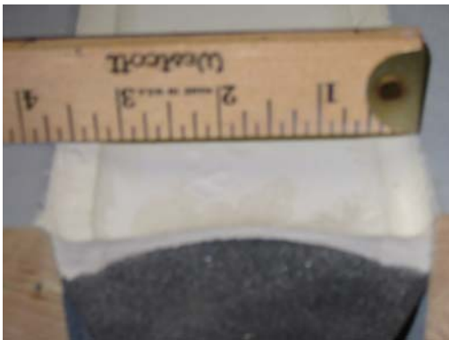
ColorJoint ESS-150 shown being tested for expansion – well beyond the published 2.25-inch capability.
