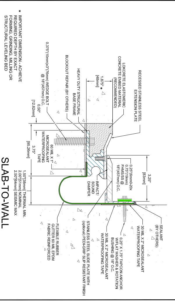
NOTE: For additional sizes refer to drawing 31350-02 for SSS-C-400, 600, 800 and 31350-04 for SSS-C-1000 EHD / SSS-C-1200 EHD
