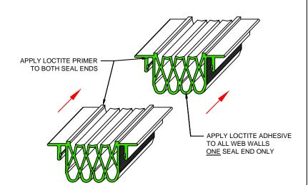
STEP 2 - Adjoin ends of seal together by applying Loctite Primer to both ends and Loctite Adhesive to only one of the ends to be joined. Hold ends together for approximately 15 seconds.
