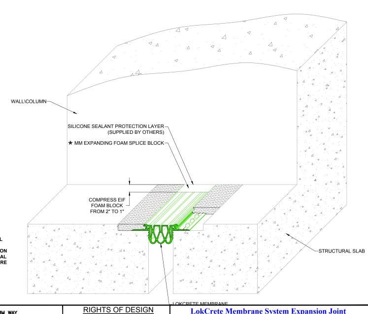
\* WARNING: THE STRUCTURAL EXPANSION JOINT OPENING IN THE DECK MUST TRANSITION INTO A VERTICAL STRUCTURAL OPENING. OTHERWISE SEVERE CRACKING MAY OCCUR.
