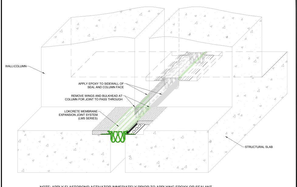
NOTE: APPLY ELASTOBOND ACTIVATOR IMMEDIATELY PRIOR TO APPLYING EPOXY OR SEALANT.
