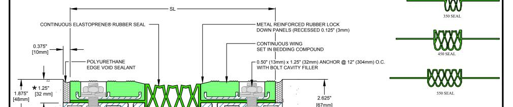
★ IMPORTANT DIMENSION - ACHIEVE REQUIRED DEPTH BY EXACT FORMING, GRINDING, MILLING OR STRUCTURAL LEVELING BED
