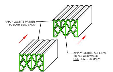
**STEP 2** - Adjoin ends of seal together by applying **Loctite Primer** to both ends and **Loctite Adhesive** to only one of the ends to be joined. Hold ends together for approximately 15 seconds.
