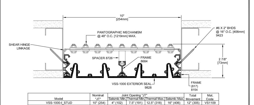
NOTE THAT EXTERIOR SEAL DISENGAGES AT 15". ( ) IN MOVEMENT TABLE DENOTES mm IN METRIC.
