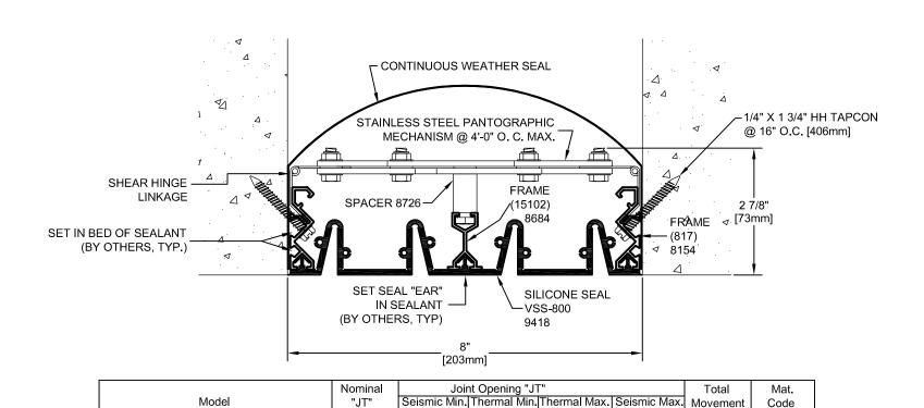
NOTE THAT EXTERIOR SEAL WILL DISENGAGE IF MOVEMENT EXCEEDS THERMAL MAXIMUM BUT WATER-TIGHTNESS WILL BE MAINTAINED BY INTERIOR SEAL UP TO SEISMIC MAXIMUM
