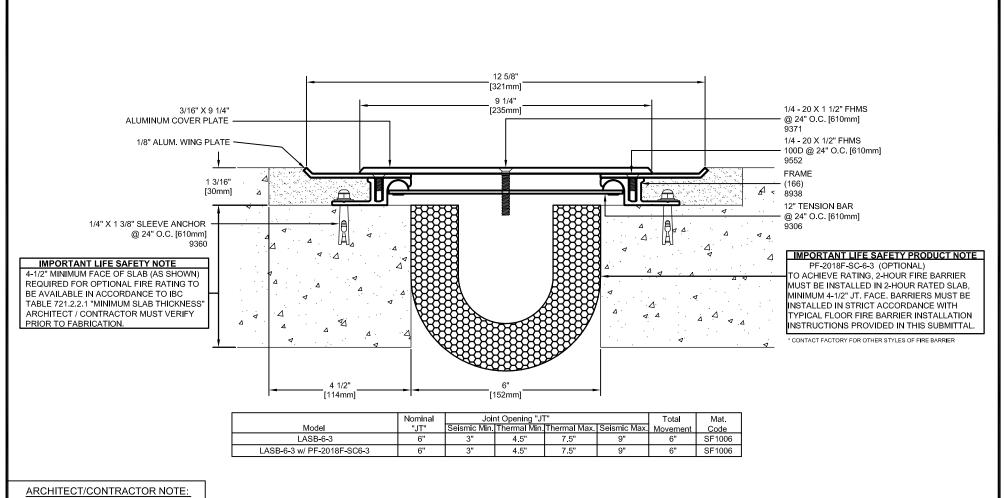
ALL SUBASSEMBLY COMPONENTS TO BE PROVIDED IN 10'-0" OR 20'-0" STOCK LENGTHS UNLESS OTHERWISE NOTED. THE SPECIFIC SYSTEMS DICTATE THE LENGTHS PROVIDED.
