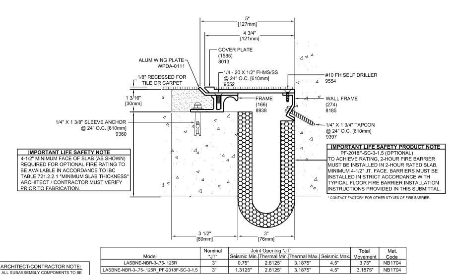
ALL SUBASSEMBLY COMPONENTS TO BE PROVIDED IN 10'-0" OR 20'-0" STOCK LENGTHS UNLESS OTHERWISE NOTED. THE SPECIFIC SYSTEMS DICTATE THE LENGTHS PROVIDED.
