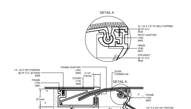
IMPORTANT LIFE SAFETY NOTE 4-1/2" MINIMUM FACE OF SLAB (AS SHOWN) REQUIRED FOR OPTIONAL FIRE RATING TO BE AVAILABLE IN ACCORDANCE TO IBC TABLE 721.2.2.1 "MINIMUM SLAB THICKNESS" ARCHITECT / CONTRACTOR MUST VERIFY PRIOR TO FABRICATION.
