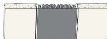
Series FSWP Wall-to-Wall / Concealed Frame Nominal Joint Openings 1" to 2"
